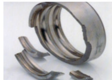
Figure 12 Forced fracture caused by a direct hammer blow.
