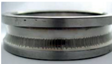
Figure 8 When electric currents pass through a bearing, there is arcing and burning at the points between the races and the rolling elements where the current jumps the air gap.
