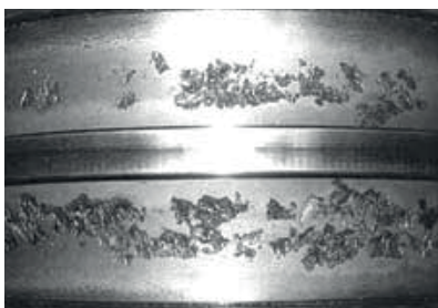
Figure 1 Fatigue spalling on the raceway
