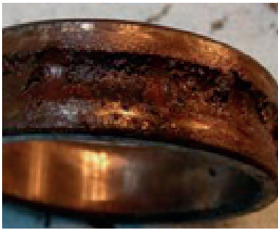
Figure 4 Rusting of a bearing inner ring caused by moisture in a lubricant
